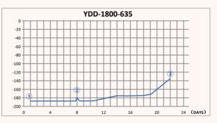
1 Precooling stage when freezer filled to high level 2 Lid open test, -179.2°C max ③ Temperature maintained below -135°C for 22 days
